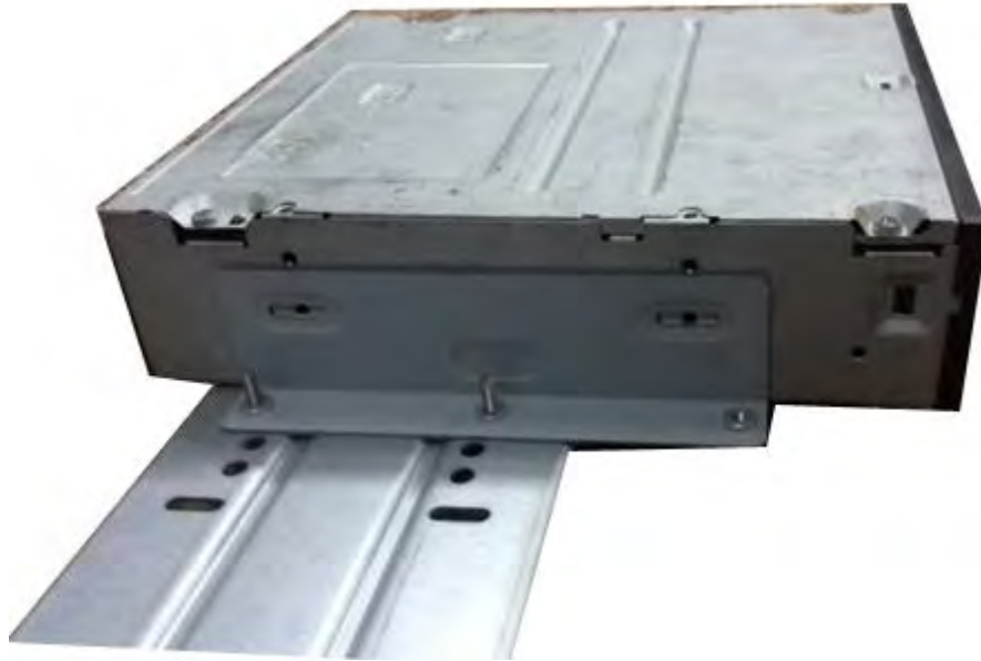
Figure 3-43 Install SATA burner
